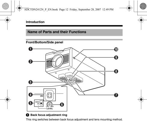
This ring switches between back focus adjustment and lens mounting method. When adjustment is required, loosen the back focus locking screw 0 by turning it anti-clockwise. After the adjustment, tighten the locking screw by turning it clockwise. This camera is factory-adjusted to a suitable position with CS-mount lens. (187 Pg. 26)
